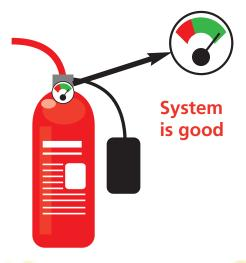
If the Firetrace® system is low on pressure due to a Fire or fault, the TraceTrace will send an SMS to the server
