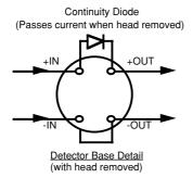
The diode must be connected so that it is shorted out by the internal connections of the head when the head is in place, and provides a path for the current in the loop when the head is removed. Incorrect fitting will not cause damage but will cause malfunctions of the system. (See troubleshooting - page 9)
