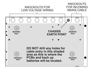
Figure 3: Semi-flush mounting diagram
