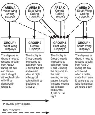
(It should be noted that, in night mode, displays not programmed to sound when a call is made will still display ALL calls on the system visually).
