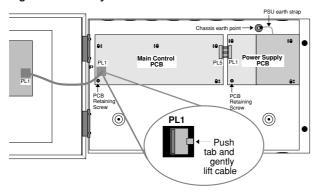
The controller <u>must</u> be sited internally in an area <u>not</u> subject to conditions likely to affect its performance, e.g. damp, salt-air, water ingress, extremes of temperature, physical abuse, etc. The liquid crystal display on the enclosure's front should ideally be situated at eye level.
